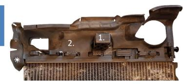
Remove electric fan with cover from original radiator by pushing down the lock tabs on the radiator and slide it out of the brackets.
