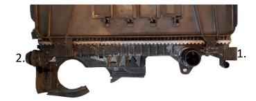
Remove air guide fasteners (1.) and air guides (2.) on both sides by twisting the air guide fastener ¼ revolution then lift it up and remove it and air guide.
