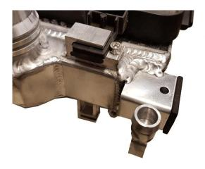
25. If installed on a manual gearbox car (without oil heat exchanger fastened to left radiator tank) block off the small 16mm connection using the included 16mm silicone cap and 16-27mm hose clamp.
