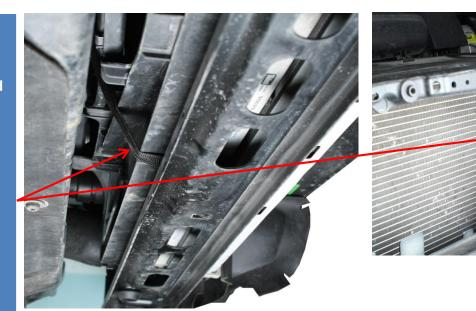
11. On both sides of the radiator support member remove 2x Hex 10mm. Remove it from the vehicle.
