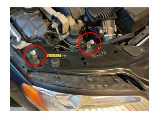
4. Remove the head lights. On both sides pull the two large metal locking pins straight up.
