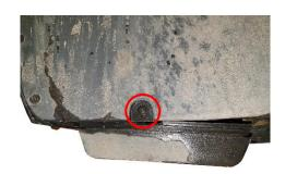
6. In the lower edge of the bumper remove 3pcs plastic rivets. Press both the plastic tabs towards the middle and then gently pull it out in its collar.
