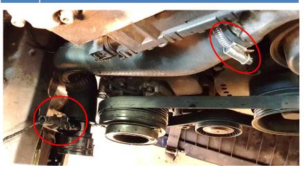
14. You may need to grind the plastic bracket slightly on the right-hand side. Keep in mind the radiators are hand build and deviation between units can occur.
