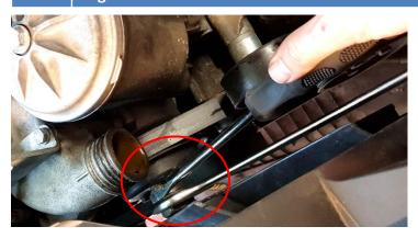
**12.** Remove 1x Torx T25 on the top left side of the radiator.
