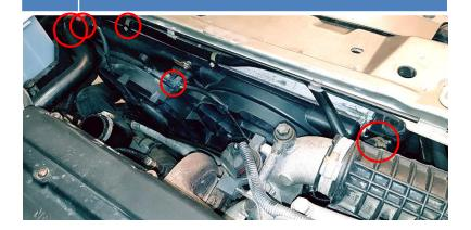
2. Remove the intercooler pipe.
