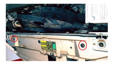
7. With the help of a strap secure the intercooler, oil cooler and AC condenser to the upper radiator support beam.
