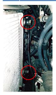
Remove 2x Hex 10mm nuts for the power steering oil cooler. (One on each side)
