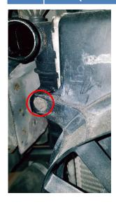
Push down both the spring loaded radiator support brackets while gently pushing the whole radiator forward (away from engine).
