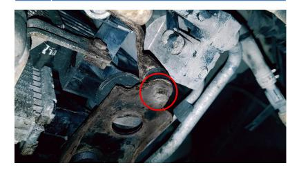
Remove 2x Hex 10mm screws for the engine oil cooler. (One on each side, screwed into the intercooler)
