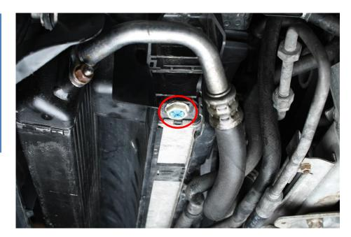
11. Remove both radiator hoses from the radiator and the small bleed hose to the expansion tank.
