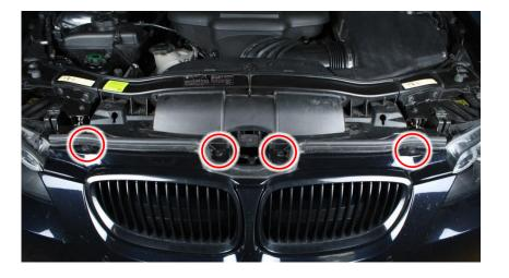
6. With help from a friend bend out the bumper on each side behind the head lights. And then pull it forward about 15cm and hold it in this position.
