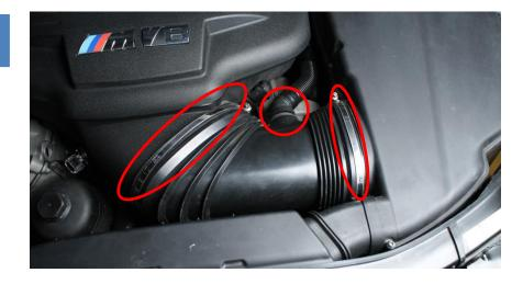
Remove 2x Torx T20 and pull out the fresh air duct to the air filter box.
