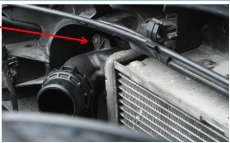
Before installing the do88 racing radiator in your car you must trim the left hand side radiator support slightly. With a small wire cutter cut away these three small plastic edges, about 5mm long. After cutting your radiator support should look like the photo.
