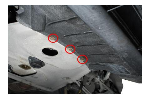
**5.** Remove the 4x Torx T30 on top of the bumper.
