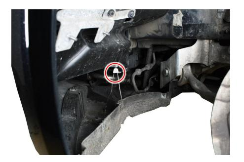
Remove 2x Hex 8mm in each upper corner of the bumper on both sides. (These become visible after you have removed the inner fenders).
