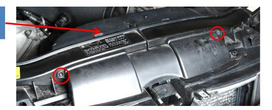
Remove 2x Hex 10mm and gently lift the entire air filter box straight up and remove it from vehicle.
