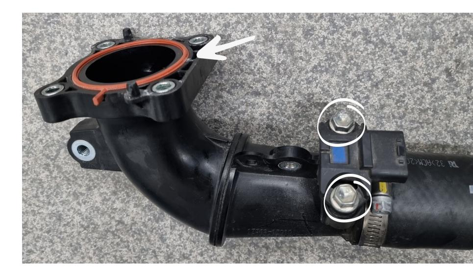
Remove the OE sealing ring and sensor and install them on do88 charge pipe using the 2x OE hex screws to fasten the sensor on the do88 charge pipe.
