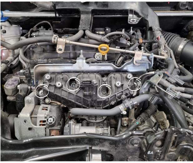
Remove 2x 10mm hex screws located at the throttle Remove 4x 12mm hex screws that holds the intake body.
