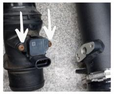
Step 10 Remove 2x T20 screws to remove the sensor.
