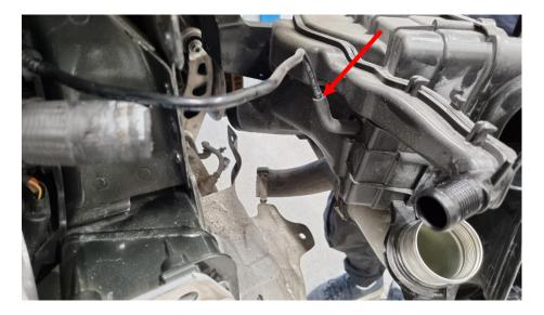
**29.** Remove the air filter box from the plastic cage. 3x metal clips.
