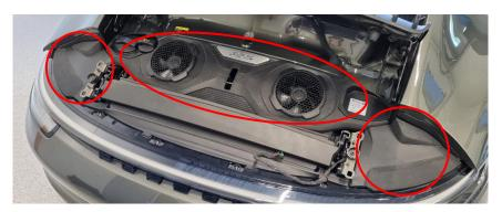
6. Disconnect the negative battery terminal. (If you skip this step, you might get fault code for the spoiler). Important! Do not close the front hood until the installation is completed and the battery terminal has been re-connected.
