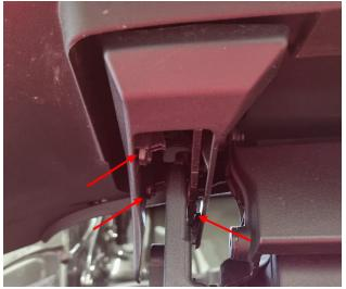
4. Remove 2x Torx T30 on each side of the spoiler mechanism. Then remove the spoiler by pulling it upwards.
