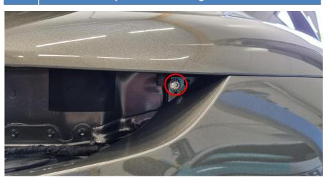
Disconnect the left and/or right cable connectors for the rear bumper. Number of connectors depends on equipment installed in the car.
