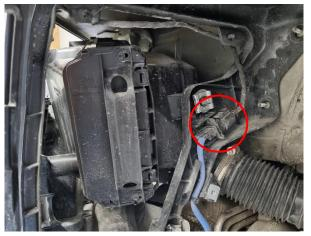
**23.** Remove the turbo inlet duct. 1x hose clamp, 1x Torx E10 (V-band), breather hose (right side only)
