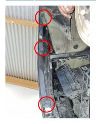
**16.** Remove the final two screws for the rear bumper cover located in the space for the rear lights. 1x Torx T30.
