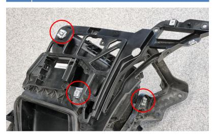
**31.** Install the do88 intercooler pipes into the air box mountings without the rubber mounting rings.
