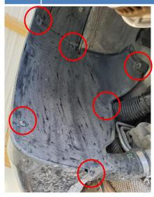
**13.** Remove 8x Torx T30 licated in the bottom of the rear bumper cover. For installation purpose, note that the two in the middle has different threads.
