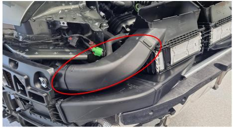
**21.** Remove four screws that holds the heat shield. 4x Torx T25.
