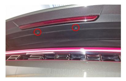
2. Remove the plastic covers underneath the spoiler. Gently pry the three locking tabs with a screw driver.
