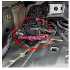
**19.** Remove the spoiler mechanism. 4x Torx T45 and 1x cable connector.
