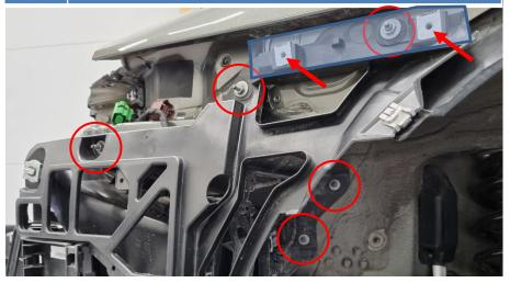
28. Now remove the entire plastic cage. On the right side you need to disconnect the vacuum line. Do this in the joint in between the plastic pipe and the rubber hose.
