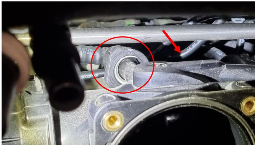
**32.** Remove the O-ring from both intake manifolds.
