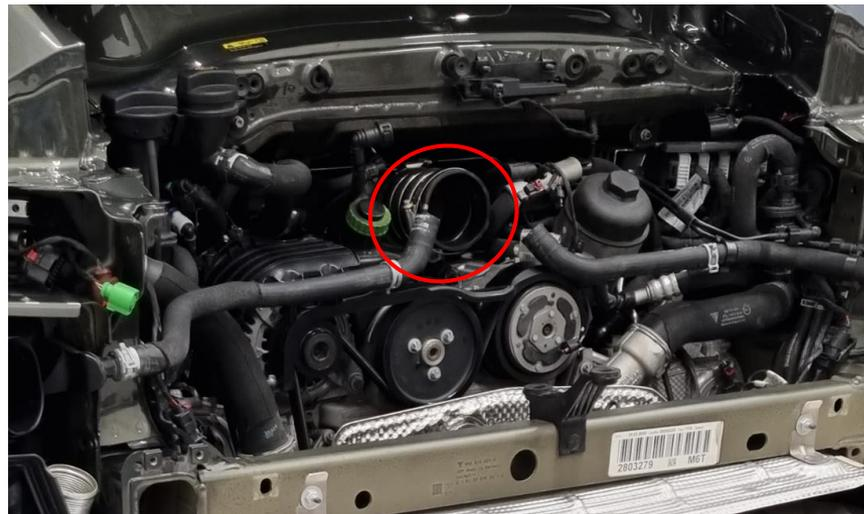
**27.** Remove the throttle body. Disconnect cable connector, 4x Torx E10 screws and 1x Hex 10mm nut.
