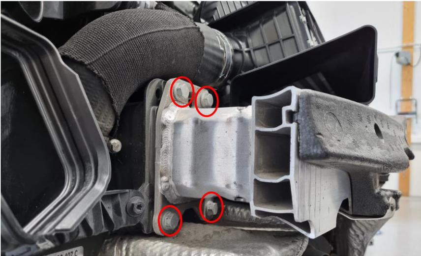
**22.** Remove the two clips and washers from the center intercooler bracket. It is a tight space to reach the front clip but can be done using two screw drivers.
