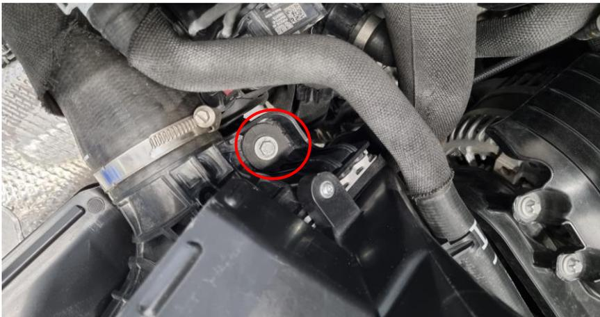
**24.** Disconnect 3x cable connector / 1x cable holder / 2 x vacuum lines / 2x rubber hoses to the BOV:s. Also loosen the hose clamp to the throttle body hose.
