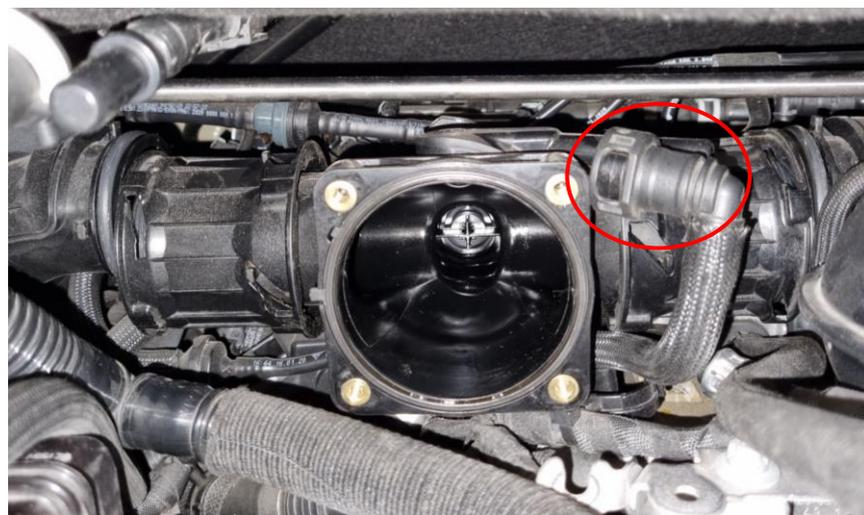
**29.** Loosen the square plastic tank and push aside to give more space. Also loosen other small ducts and parts that will give more room around the plenum.
