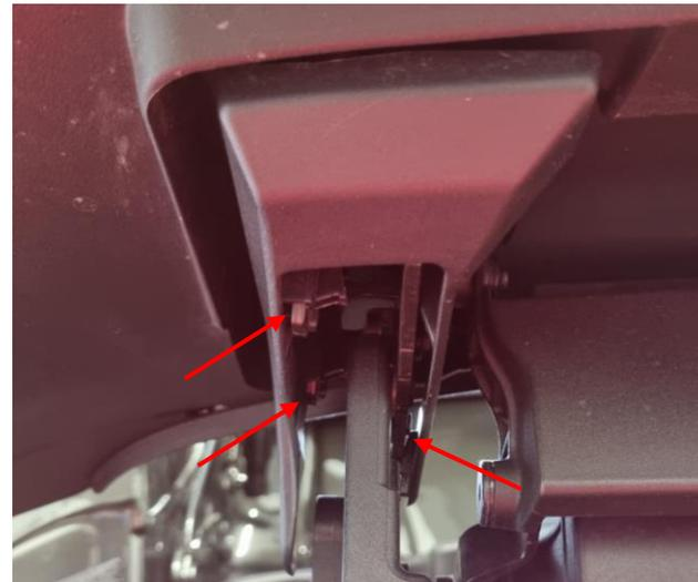
3. Remove the brake light from the spoiler. Gently push a short flat screwdriver into the holes in the two marked positions and pry the light loose. Disconnect the cable and separate the cable and grommet from the spoiler.
