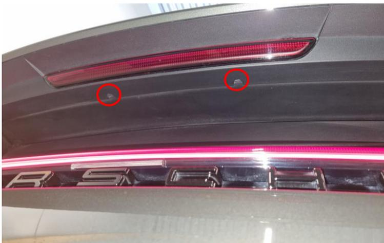
4. Remove 2x Torx T30 on each side of the spoiler mechanism. Then remove the spoiler by pulling it upwards.
