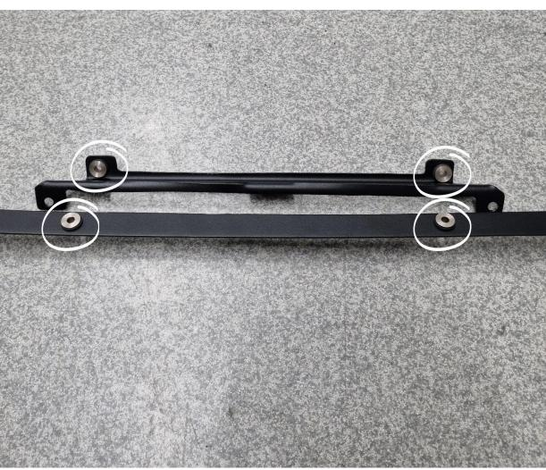
Install 4x rubber grommet in both oil cooler brackets.
