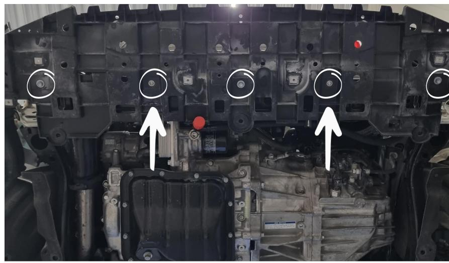
Remove the plastic cover underneath the radiator. 5x 10mm Hex screws.
