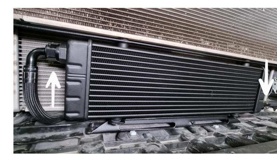
Tighten the oil hose fittings to the oil cooler with a wrench until the metal surfaces meet or maximum to 29.5 lb.-ft. (40 Nm). When tightening these fittings, it is important to hold a wrench on the hex flange on the oil cooler, so it won't get damaged.
