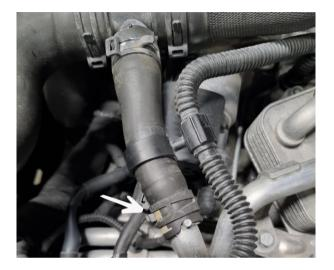
Loosen the spring hose clamp from the coolant pipe and rotate the clamp downwards to make sure it does not interfere with the air filter box.
