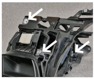
Step 22 Remove the air filter box from the plastic cage. 3x metal clips.
