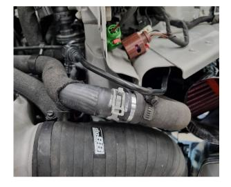
Reinstall the air filter cage in the car, fasten it with the 5x Hex 10mm nuts removed in step 19. Push on the turbo outlet hose without tightening the clamp yet.
