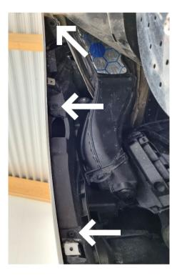
Remove 8x Torx T30 screws located in the bottom of the rear bumper cover.
