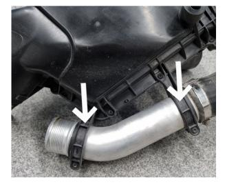
Step 24 Remove the charge pipe from the OE air filter box. 2x Torx T25.
