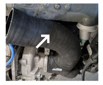
Install the inlet hose. Tighten the included 60-80mm / 9mm wide hose clamp loosely so the hose still can rotate on its connection.
