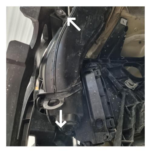
Remove the frontal fresh air ducting connected in-between the air filter box and the rear fender air intake. 1x Torx T30 screw at the top and 1x plastic tab at the bottom. Loosen screw and press tab while pulling the air ducting downwards.
