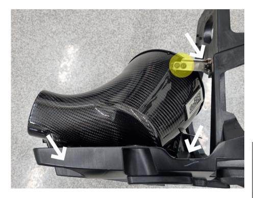
Install the do88 air filter box in the plastic cage. It is fastened in 3 locations, the hole you drilled in step 23 and in two of the OE fastening locations (rubber bushings). Use these parts from the included hardware:
