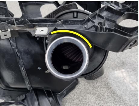
Install two of the included silicone hoses and aluminum joiners (photo above shows the right side).
