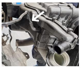
Now remove the entire plastic cage. On the right side you need to disconnect the vacuum line. Do this in the joint in between the plastic pipe and the rubber hose.
