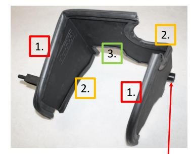
**3.** Install the lower rubber bushing on the heat shield and the upper rubber busing in the car.
