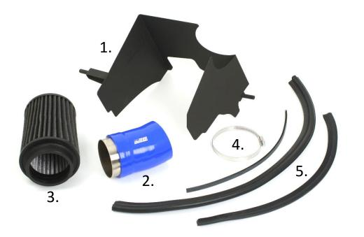
This instruction shows how to replace the OEM air filter box with do88 performance air inlet.
