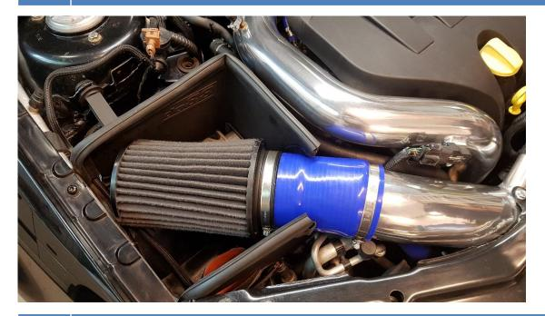
Push on the silicone hose onto the air intake pipe. Then push on the air filter onto the metal sleeve on the silicone hose. Adjust the rotation on the silicone hose into a good position before tightening the hose clamps.
