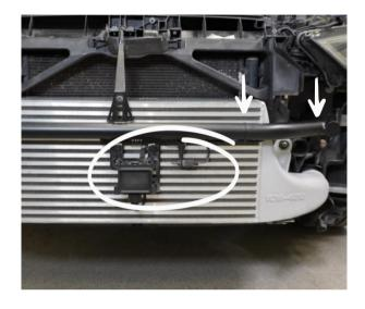
(8V only) Install the ACC and outside temperature sensor.
