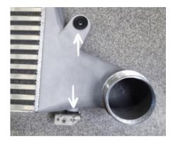
Remove the bushings and brackets from the OEM intercooler and install it on the do88 intercooler in the same positions as mounted on the OEM.
