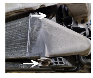
Remove 3x Torx T25 and disconnect the cable clips along the crash bar.
