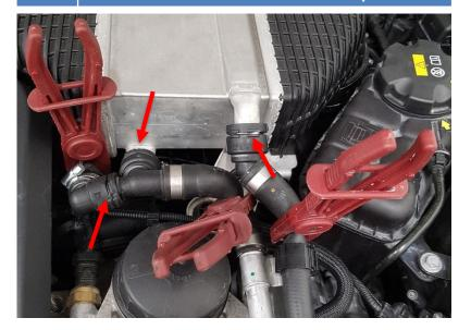
5. Disconnect the plastic hose from the intercooler bracket.
