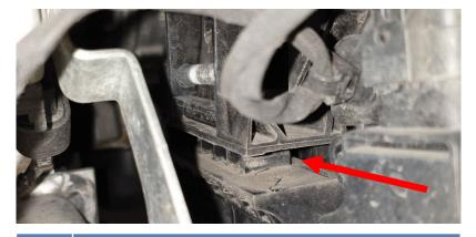
**19.** Use an angled pry tool from the backside of the intercooler air guide to separate it from the locking tabs then lift it off the hooks and remove.
