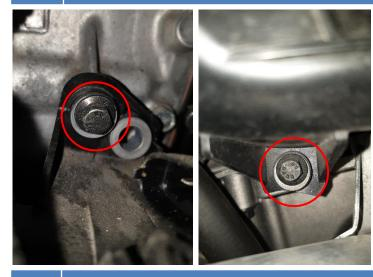
**15.** From both intercooler connections and turbo outlet, remove clips the way described in step 8 and then remove these three hoses.
