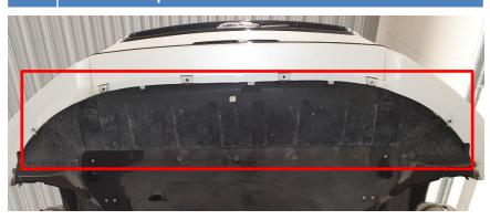
6. In the lower left corner of the bumper, separate the electrical connectors from the bottom plastic so they are loose from it.
