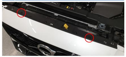
**9.** From the top of the bumper, remove 5pcs Torx T25 marked in red.
