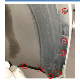
7. Loosen the bottom plastic part just behind the bumper. If needed to remove completely to gain access it might be necessary to cut a few cable ties that holds cables on top of it.
