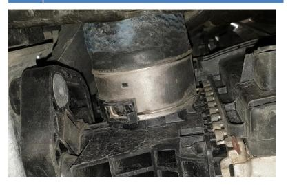
14.With both pipes loose, now remove the upper<br/>pipe from the hoses to make space for removal of<br/>lower pipe.<br/>Then remove the lower intercooler pipe from its
