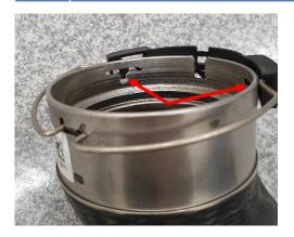
20. Install the sealing ring and lock clips in the included Henn connector adapters. Make sure the sealing ring is installed in the same direction as it was in the OEM hose.
