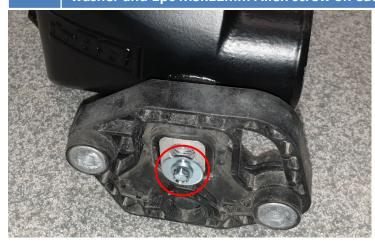
22. Remove both intercooler mounts from intercooler by prying locking tabs seen from bottom of intercooler using a screwdriver then remove locking plates and slide mounts off the intercooler.
