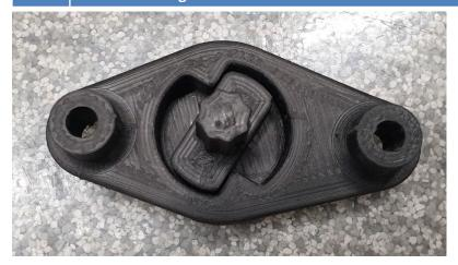
**33.** Assemble the actuator to the grille shutter limiter with the T-shaped rotation limiter as close as possible to the rotation just determined. Secure with 2pcs 5x25 screws included, screw in slowly to avoid damages to the actuator housing.
