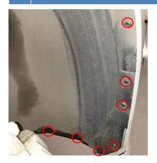
**3.** In the lower edge of the bumper remove 3pcs plastic rivets. Press both the plastic tabs towards the middle and then gently pull it out in its collar.
