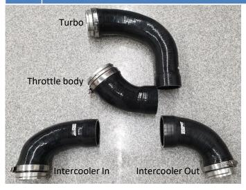
23. Install upper intercooler pipe in hoses and fasten it using 2pcs included M8x20 hex head screws. Install hose clamps and tighten them.
