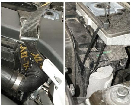
Loosen the fan cover by pressing in the locking tabs on both sides, then lift the fan cover about 2cm (3/4") upwards. Leave it in this position.
