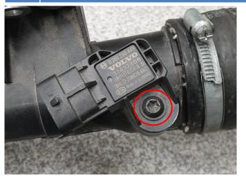
**17.** Install sensor in do88 intercooler pipe and secure with supplied M5x12 Flange screw
