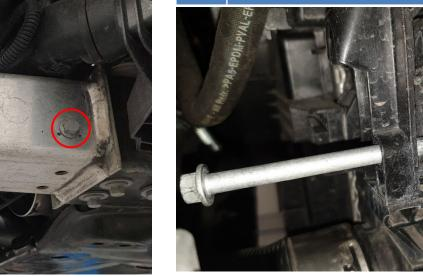
Pry here with a screwdriver to separate the intercooler. Then remove intercooler from car by first lowering the right side until the left side slides out of its bracket. Be aware of the lower left fan cover bracket so you don't damage it.
