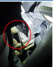
**14.** Loosen intercooler air guide from the intercooler by pressing in the locking tabs and then lift the air guide a bit upwards.
