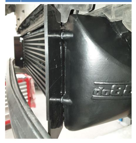
**30.** If car have active grille shutter follow step 30-34: Note the position of the active grille shutter and keep it in this position. Remove two Torx T20 and then remove actuator from shutter.
